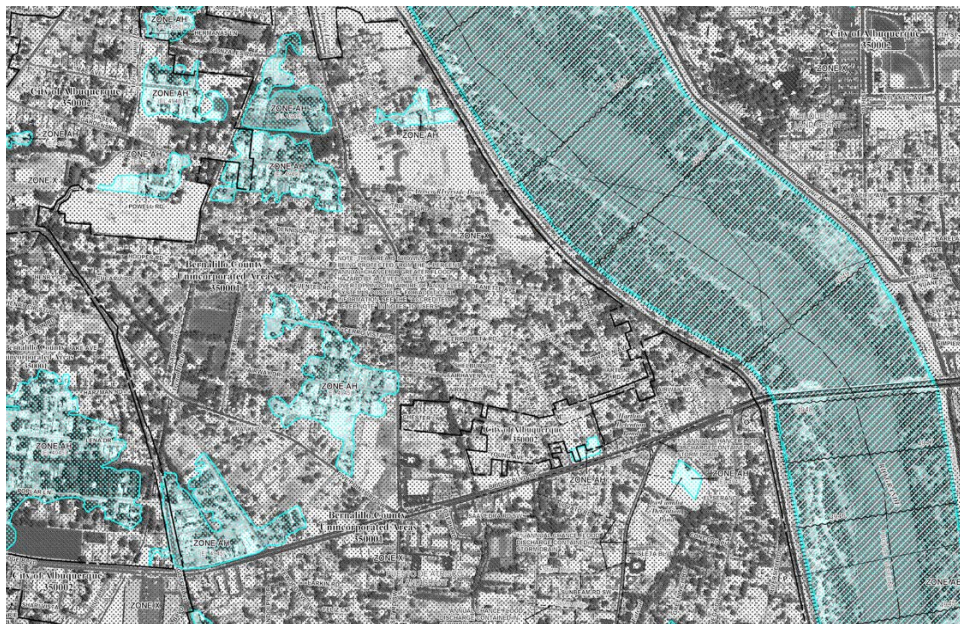
Figure 15: Example of local flood risk as determined by FEMA for a portion of Downtown Albuquerque. Blue shaded regions are the 1% annual flood risk areas (Zone AE & Zone AH) FEMA Flood Insurance Rate Map – Bernalillo County, Panel 333 of 385 Map
